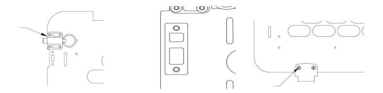
7. Attach the base plate (1) to the hinge blade (3) using the stainless steel pin (2).
