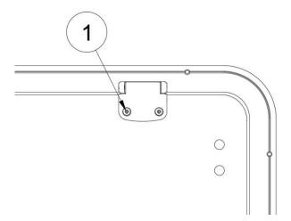
23. When installing an Explore Overlander on a sliding window, replace the top screw of the spring latches with the supplied M5  $\times$  20 socket head cap screw (1). This screw is covered with a plastic cover.
