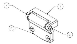
6. Mount the hinge blades (2x), spring latches (2x) and the protection plates (2x) with the accompanying screws on the Overlander.
